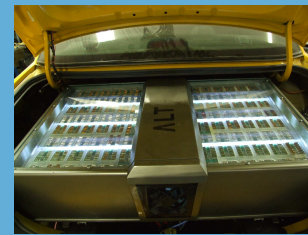
Gen 1 Series PHEV Powertrain in a running Ford Crown Victoria
